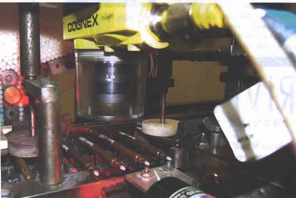
This vision system uses LED lighting to inspect felt-tip pens. Photo courtesy Cognex Corp.
